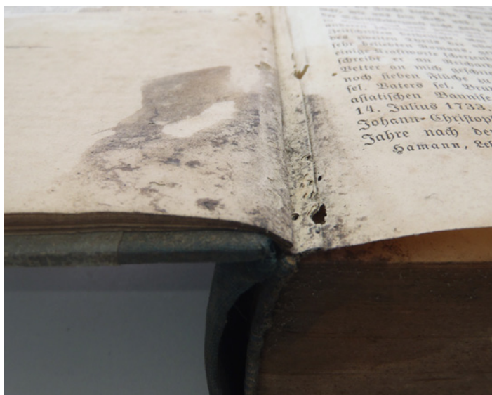
Fig. 1: Book contaminated by darkly pigmented fungal mycelium and damaged by insects.
