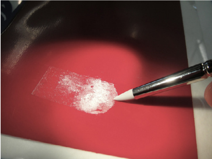
Fig. 4: Removal of the tapes adhesive residues with cellulose powder and a color shaper tool
