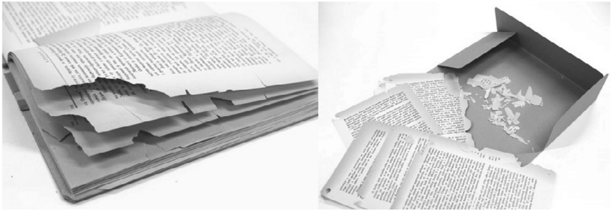
Fig. 3: The consequence of 50 instances of handling for the paper (bound and unbound) with the lowest DP.
