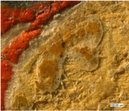
Fig.1: Prudentius 9. Jh., Burgerbibliothek Bern, Cod. 264, 2, p.18 detail: a drop of petrolatum lays on the surface.
