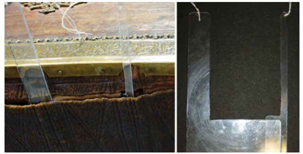
Fig. 4: Vivak templates for supporting the spine leather and linen glued together to press it while drying
